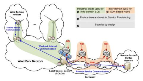
Figure 2. VirtuWind architecture and requirements.
