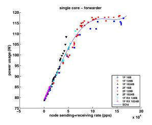
Figure 1. Power consumption as a function of packet rate for a single core router and for different packet sizes (16, 128, and 1024 Bytes) [11]
