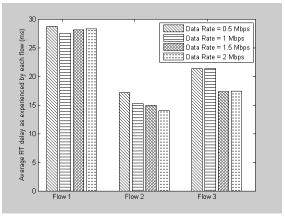
(b) Routing based on delay
