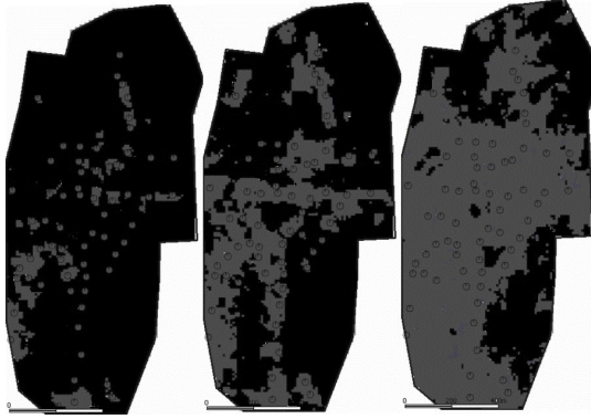
Figure 8.5: Uplink coverage of the Femto-Baseline (left), Pico-Baseline (middle) and DUDe (right) cases where black and grey represent the MCells and SCells coverage respectively.
