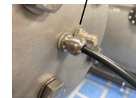
high-pressure cable gland
