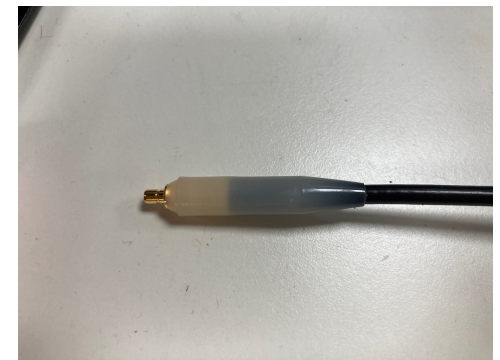
Over-moulding of RG174 (w/ SMB connectors)
