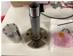
High-pressure pipe and flange
