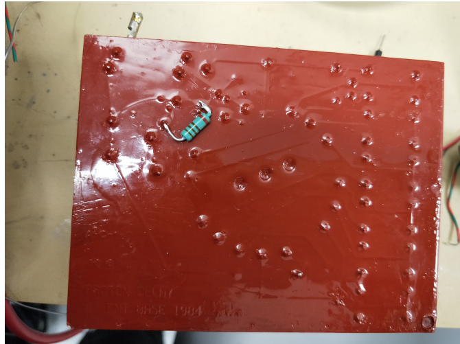
fig.8. 110\Omega resistor multiple to control the whole resistance of base circuit.
