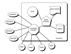
Fig. 1: The architecture of JCAT.
