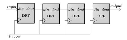
Figure 7: A simple shift register
