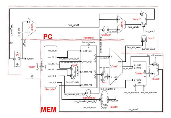
Figure 13: A Schematic View of the Single-Cylce mMIPS Design
