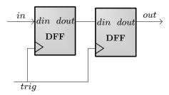
Figure 9: A two bit shift register
