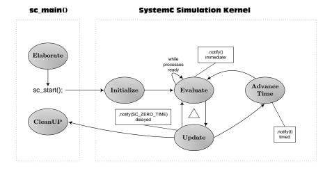
Figure 2: SystemC Simulation kernel ([4])
