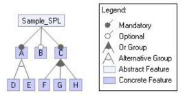
Figure 1: The feature model of a sample SPL
