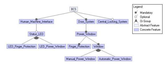
Figure 4: The feature model of a simplified version of the BCS SPL (inspired by [29])
