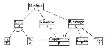
Figure 3. Feature diagram of the vending machine [7].
