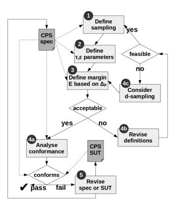
Fig. 2. Process for sound conformance testing
