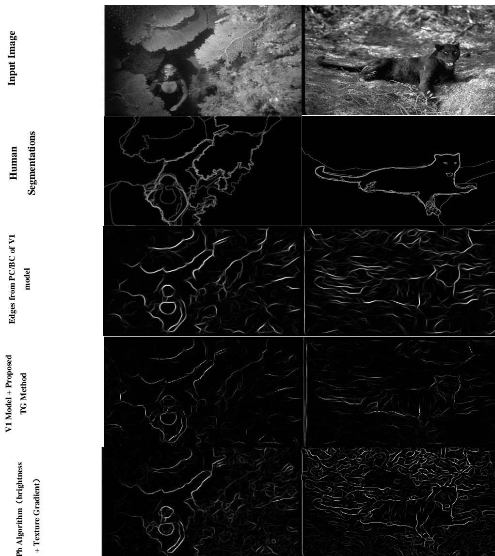
Figure 7 Two Images from BSDS300 Dataset [9] and Their Image Segmentation Results Obtained by Different Algorithm
