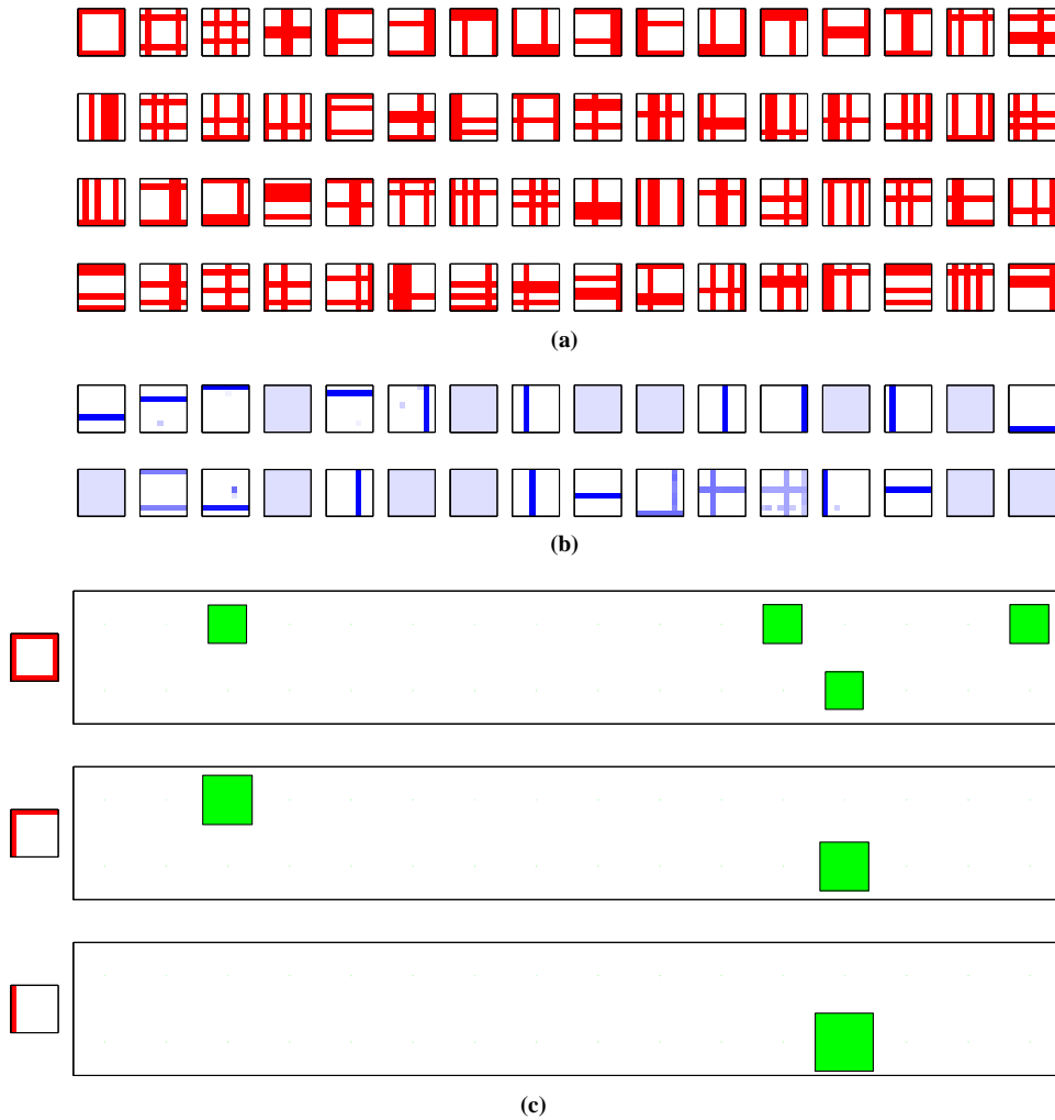
Figure 8: A network generating a distributed code for four bar patterns. (a) Training data consisting of 64 images each on an 8 by 8 grid of pixels. Dark pixels indicate active inputs. (b) The synaptic weights for the 32 nodes in a network after training for 1536 cycles. Each box represents the weights learnt by an individual node. The darkness of the pixels within each box corresponds to the strength of that weight. (c) The response of the network, after training, to three test patterns. The left-most column shows the input pattern, with the remainder of each row showing the response of the network to this pattern. The size of each square corresponds to the strength of the response of each node. Responses are shown in the same order as the weights are shown in (b). This network generates a distributed code in response to one of the training patterns and a local code in response to an isolated bar feature.
