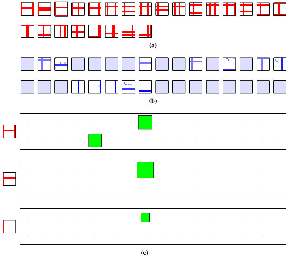
Figure 6: A network generating a distributed code for three bar patterns based on nodes selective for different sub-features to figure 5. (a) Training data consisting of 24 images each on an 8 by 8 grid of pixels. Dark pixels indicate active inputs. (b) The synaptic weights for the 32 nodes in a network after training for 768 cycles. Each box represents the weights learnt by an individual node. The darkness of the pixels within each box corresponds to the strength of that weight. (c) The response of the network, after training, to three test patterns. The left-most column shows the input pattern, with the remainder of each row showing the response of the network to this pattern. The size of each square corresponds to the strength of the response of each node. Responses are shown in the same order as the weights are shown in (b). This network generates a distributed code in response to one of the training patterns and a local code in response to certain pairs of bars and also to certain isolated bar features.
