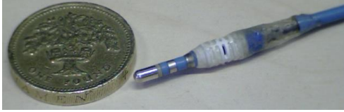
Fig. 2. Photograph of the prototype fiber-optic sensor integrated with a 7 Fr catheter. A one GB pound coin is shown for comparison.
