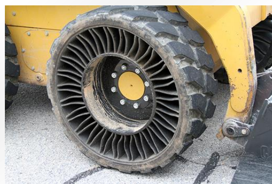
Figure 4: Michelin Tweel, Source: Construction Business Owner [5]
